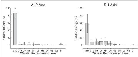
**Figure 2 Axial energy contribution from wavelet decomposition**. Relative energy contribution from each wavelet decomposition level in each axis, averaged over all swallows from both discrete and sequential tasks. Vertical and error bars represent means and standard deviations, respectively.
